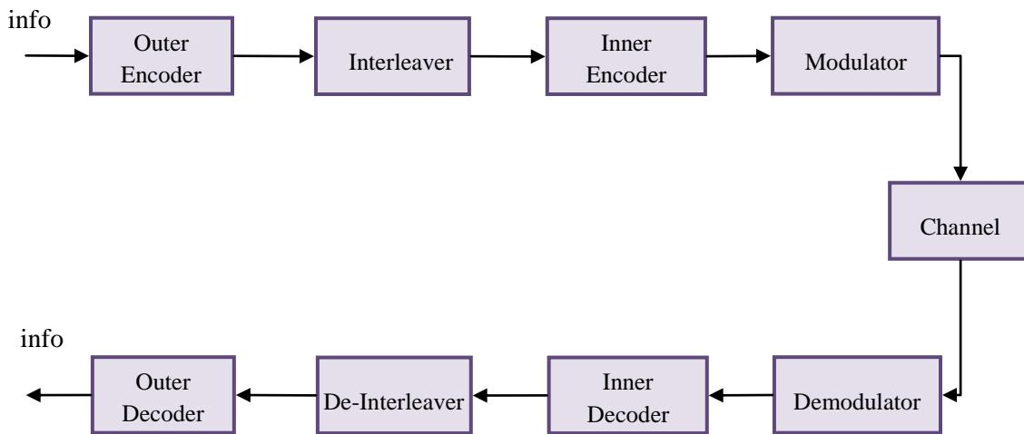
Fig 1: Block diagram of Concatenated codes
