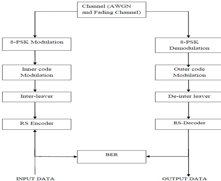
Fig 2 : Concatenated BCH and TCM with 8PSK modulation
